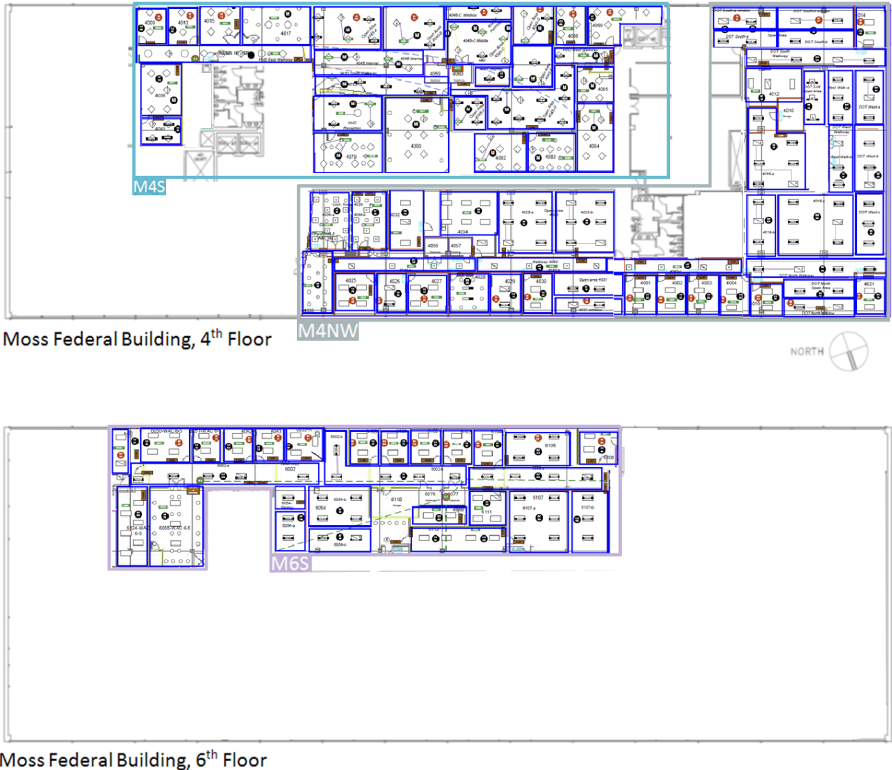
Figure 12: Moss post-retrofit lighting control zones
