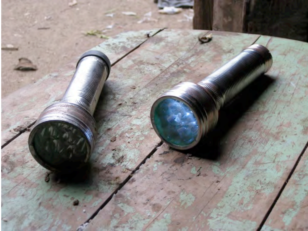
Photo 2. LED flashlights used by a household that requires two dry cell D batteries.
