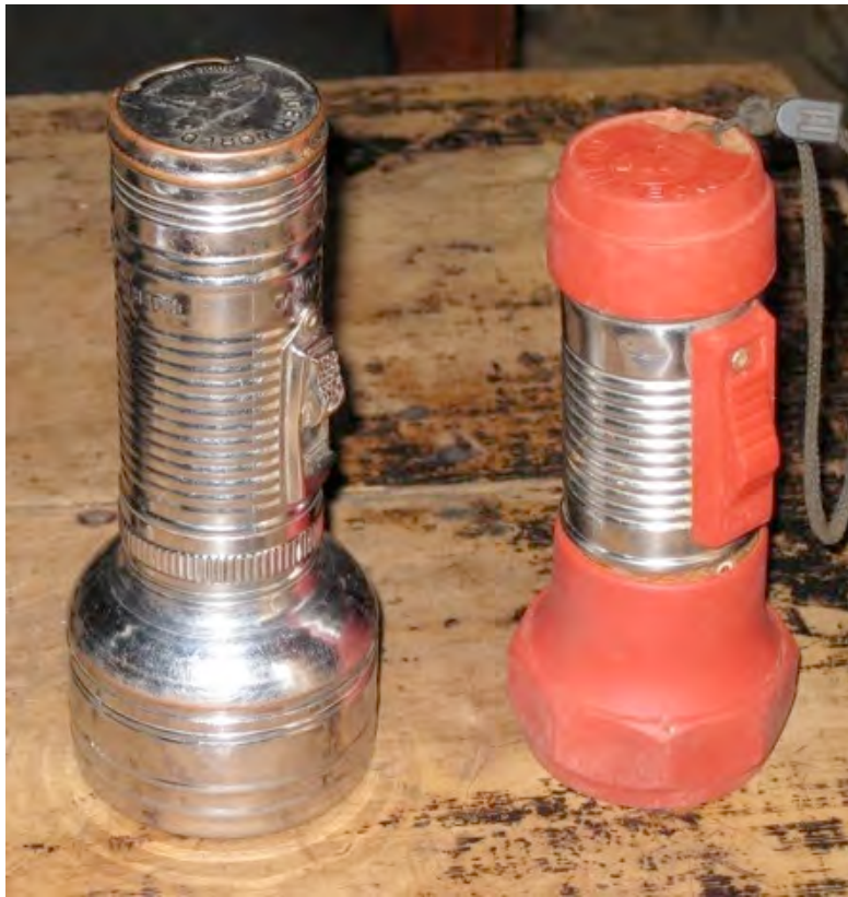
Photo 3. LED flashlights used by a household that requires only one dry cell D battery.
