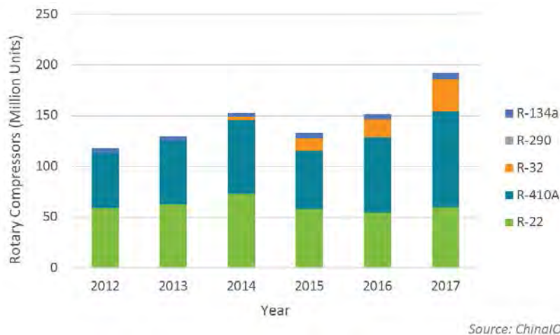
Figure 2.6: Chinese Production of Rotary Compressors by Refrigerant, 2012-2017 (Nicholson and Booten, 2019). Note: HFC-134a rotary compressors are primarily used in mobile cooling applications, in contrast to the rest of the rotary compressor market which is used mainly for room (stationary) air conditioning.
