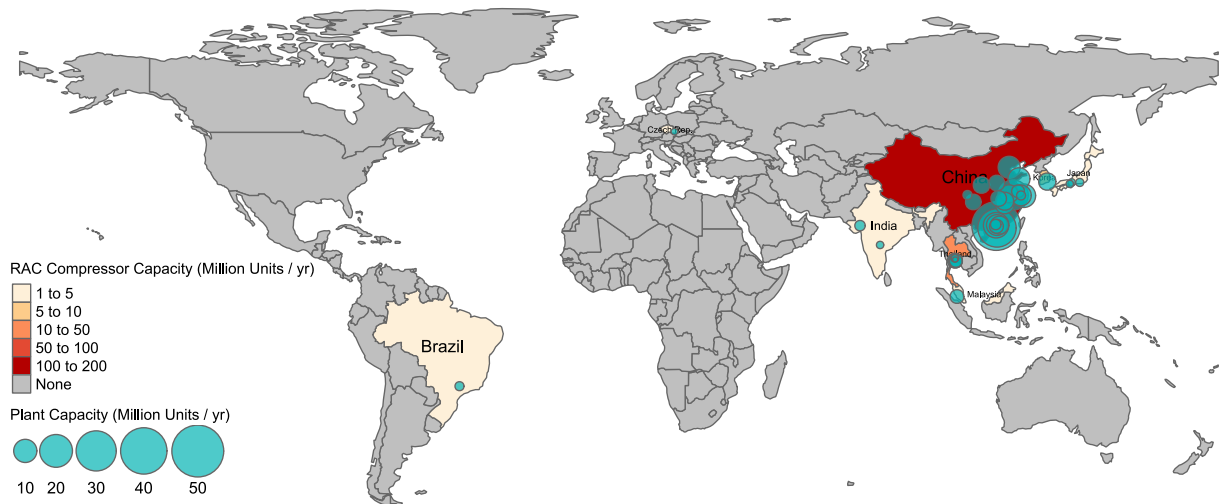
Figure 2.4: Global RAC Rotary Compressor capacity as at September 2018 (Nicholson et al 2019)
