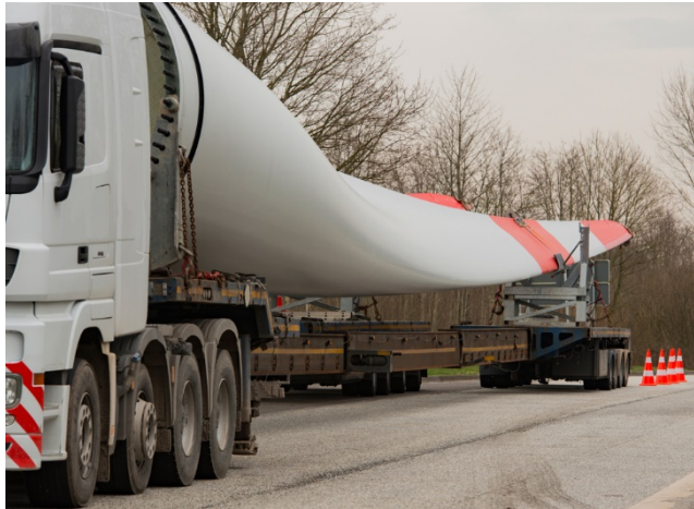
Figure 2-14 Ground transportation of blade
