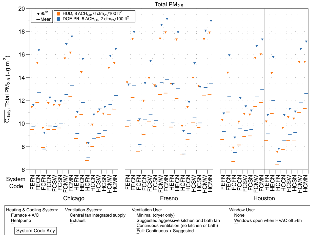
Figure 21 Simulation results for mean and 95 th percentile daily concentrations of indoor PM 2.5 from all sources.
