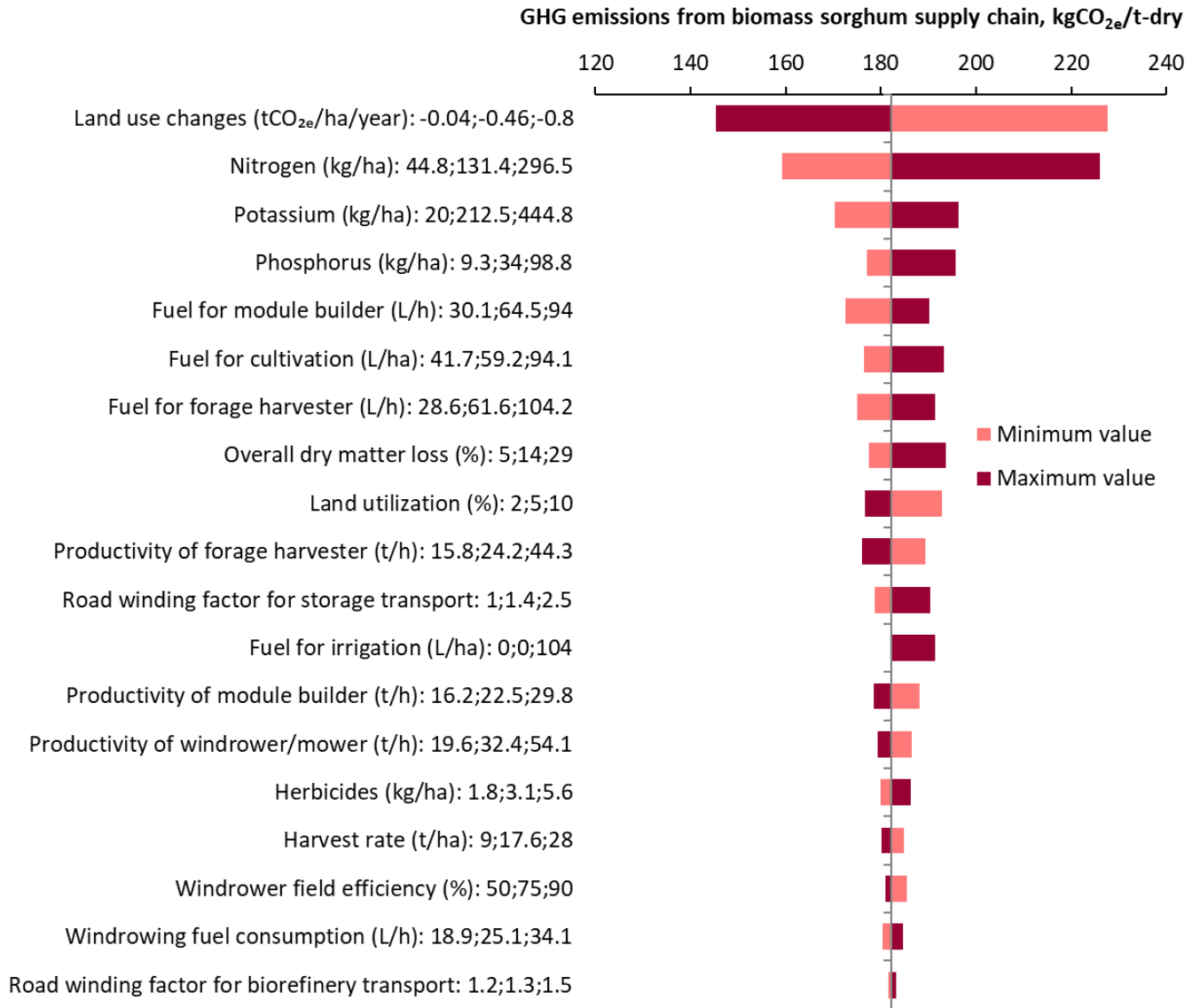
Figure S24. Sensitivity to the GHG emissions for the biomass module supply system with preprocessing depot. t = metric ton.
