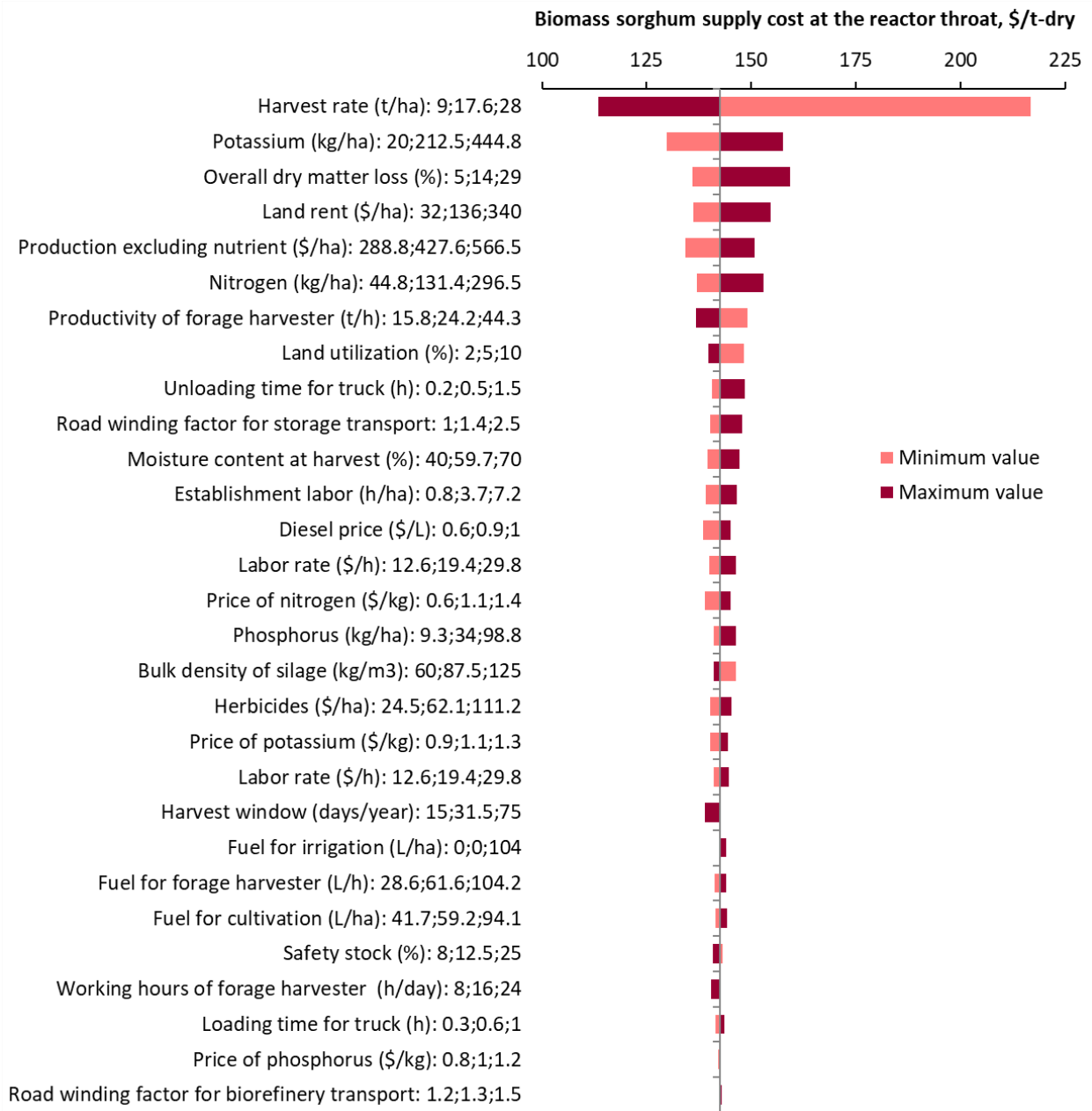
Figure S4. Sensitivity to the biomass feedstock supply cost for the chopped ensiled biomass supply system with preprocessing depot. t = metric ton.
