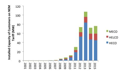
Figure shows net energy metering installations in MECO, HELCO, HECO (Hawaii) from 2001 to 2015. In five years customers install 246 MW, 54 MW and 58 MW, respectively, of NEM DG (22%, 29%, 30% of 2013 system peak).
