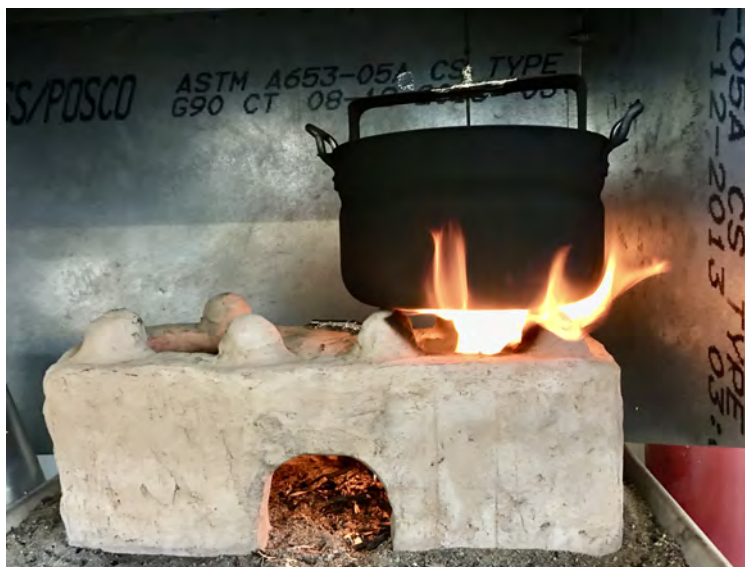
Figure 5.3: Two-pot mud chulha in use at LBNL Cookstove testing facility.
