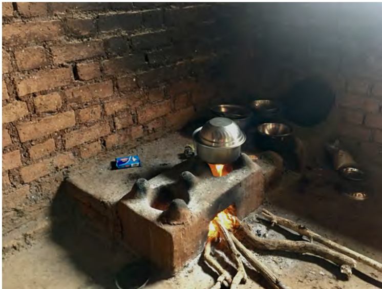
Figure 4.3: Baseline mud chulha stove found in Maharashtra, India. The mud chulha shown is 2-pot design.
