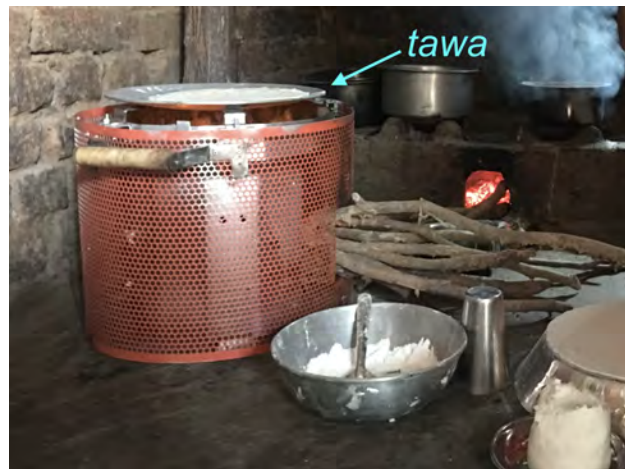
Figure 2.7: Side-view of Berkeley-India Stove (final version/version 2) in use in a household in rural Maharashtra.
