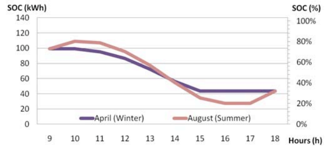
Fig. 5. Operation schedule of PEV batteries for two example months.
