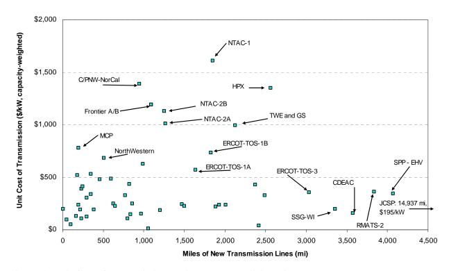
Figure 6. Unit Cost of Transmission vs. Added Transmission Distance
