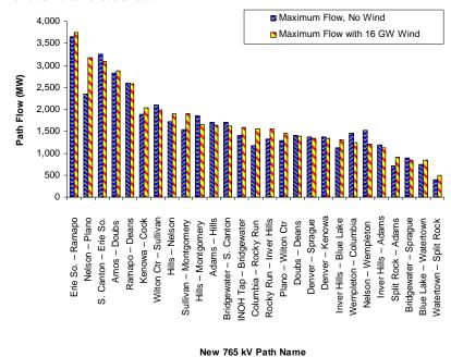
Figure 4. Maximum Power Flow on 27 New 765 kV Paths With and Without 16 GW of New Wind Generation in the MISO '06 Study (MISO 2007)
