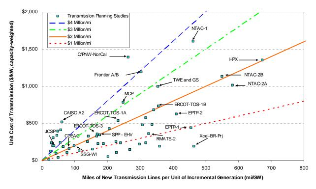
Figure 7. Unit Cost of Transmission vs. Added Transmission Distance per Unit of Incremental Generation
