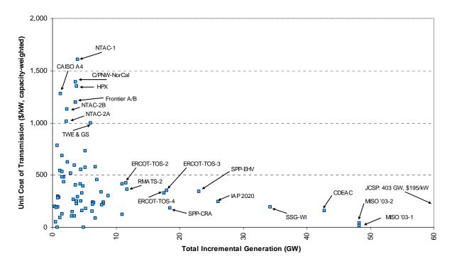
Figure 5. Unit Cost of Transmission vs. Generation Capacity Additions
