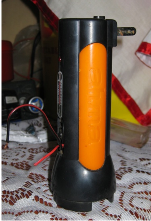
Photo 5. A Household flashlight that had a failed switch and was rewired by the user.
