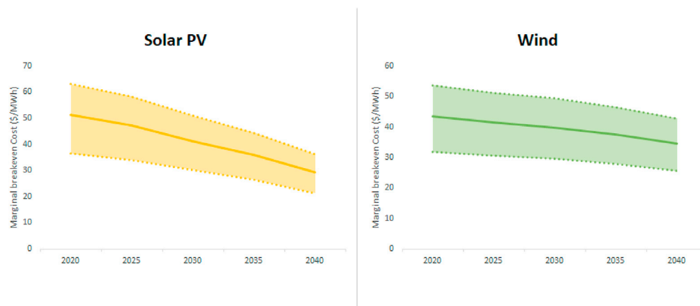
Figure 5. Implied marginal breakeven costs (2018 US$/MWh) for solar PV and wind relative to new coal generation, LDHR scenario
