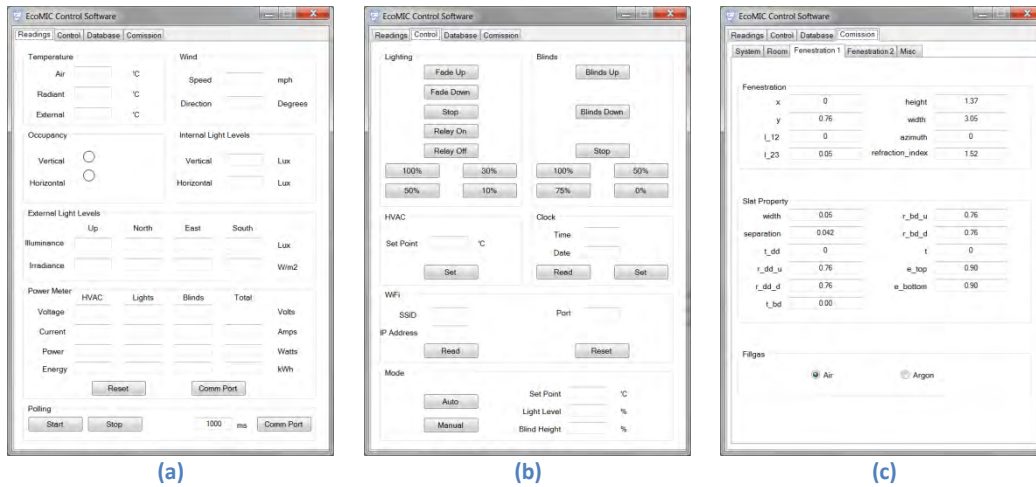
Figure 40 EcoMIC VBA tool example: (a) monitoring page (b) control page (c) commissioning page.
