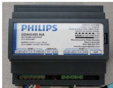
Figure 35 DDNG485 network communication gateway.
