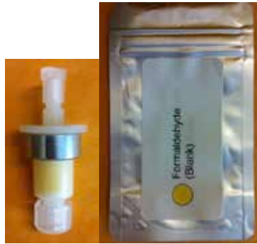
Formaldehyde sampler BLANK inside airtight bag
