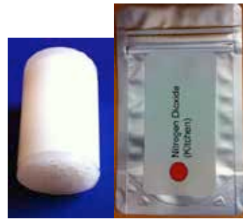
Nitrogen dioxide sampler inside airtight bag
