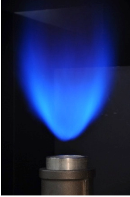
Figure 6. The lifted flame produced by the low-swirl burner
