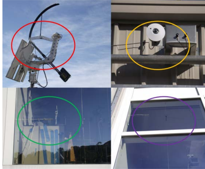
Figure 12 Instrumentation used at the test facility (Pyranometer (top left), pyrgeometer (top right), temperature sensors (bottom left), pyranometer (bottom right))
