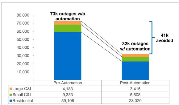
Figure 6: Comparison of Number of Outages With and Without Automation (For an Extreme Weather Event on July 5, 2012)
