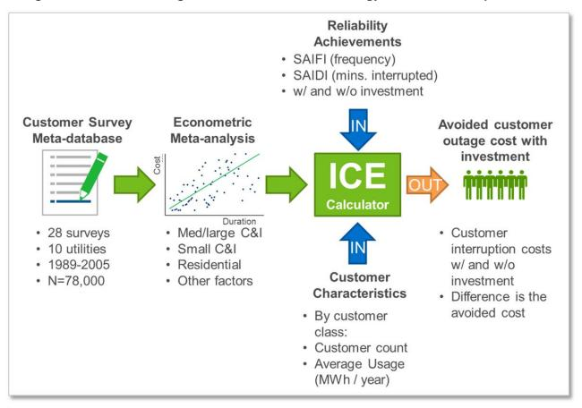
Figure 2: Customer Outage Cost Estimation Methodology under Normal Operations
