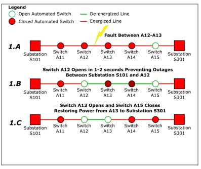
Figure 1: Outage Mitigation and Restoration Example for a Single Feeder Circuit
