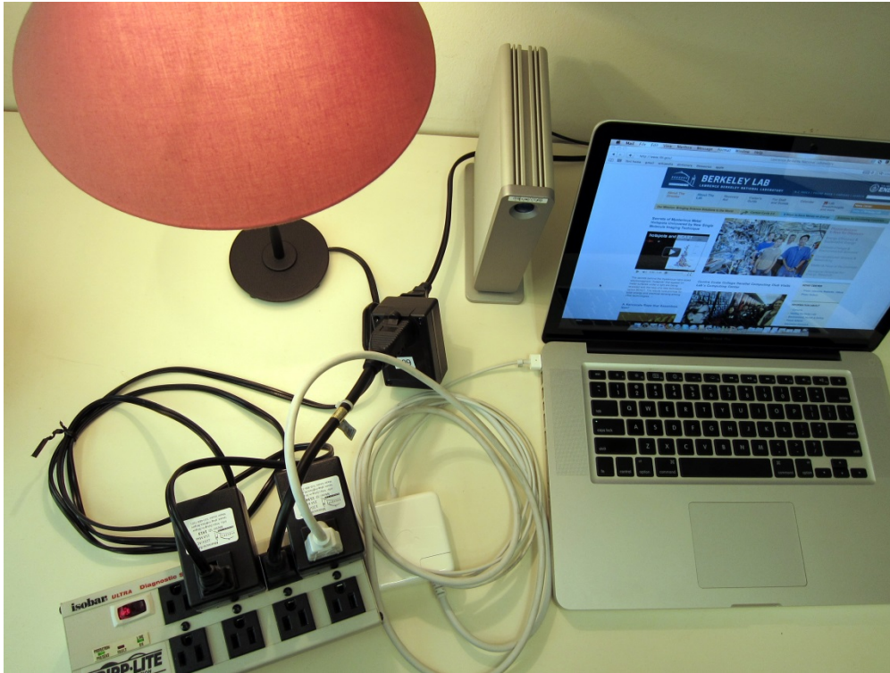
Figure 3 ACme devices metering loads
