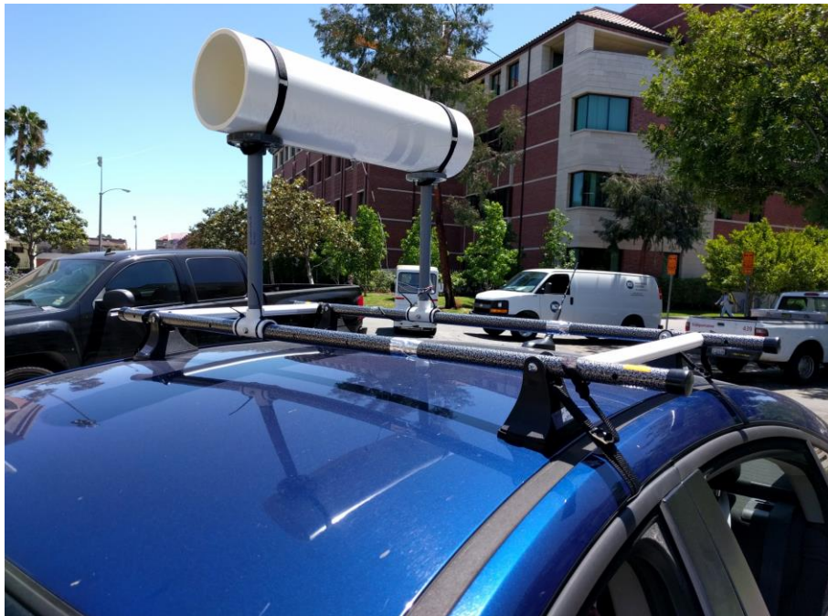
Figure 5: Mobile Monitor on Quick-Install Car-Roof Mount
