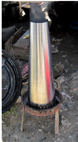
Figure 1 – Example of a lighting cone on a traditional Haitian sheet metal stove. A lighting cone is used to decrease the ignition time of a charcoal bed.
