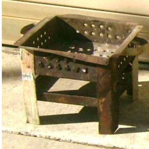
Figure 3 – Traditional Haitian charcoal stove used for testing. Stove dimensions: height = 270 mm, length/width = 110 mm, weight = 2.8 kg
