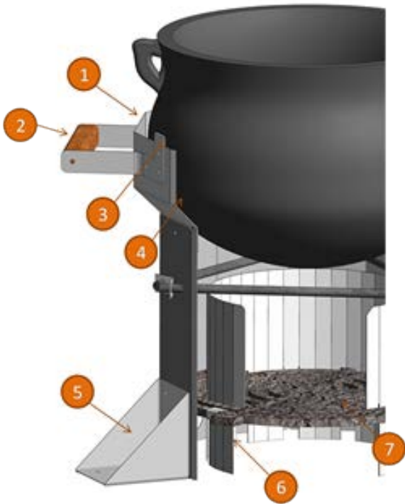
Figure 1. Schematic of the Berkeley-Darfur Stove. (1) A tapered wind collar that increases fuel-efficiency in the windy Darfur environment and allows for multiple pot sizes; (2) Wooden handles for easy handling; (3) Metal tabs for accommodating flat plates for bread baking; (4) Internal ridges for optimal spacing between the stove and a pot for maximum fuel efficiency; (5) Feet for stability with optional stakes for additional stability; (6) Nonaligned air openings between the outer stove and inner fire box to accommodate windy conditions; and (7) Small fire box opening to prevent using more fuel wood than necessary.
