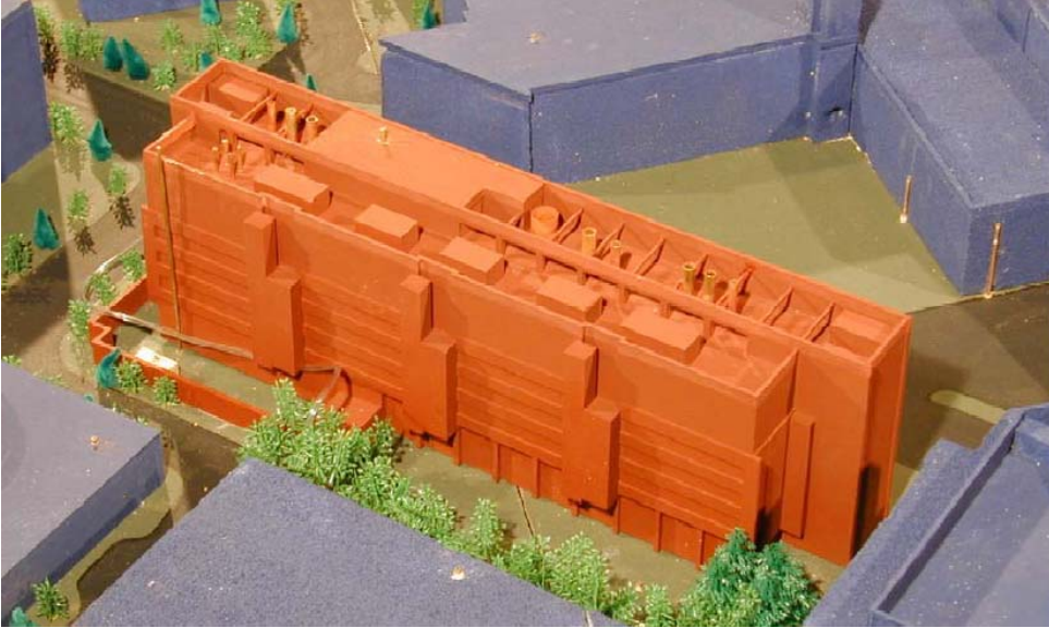
Figure 1. This wind tunnel model for a medical research laboratory in an urban environment showed that stack configuration was inadequate, even with an entrained air stack. Source: Cermak Peterka Petersen
