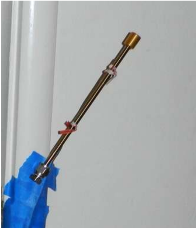
Figure 6: A stainless steel desorption tube passive tracer gas sampler as installed. The sampler is attached to the end of the copper tubing inlet to the active sampler, which is directly behind the desorption tube in the image. The cap is attached to the lower left side of the tube and the protective cap is on the upper right side.
