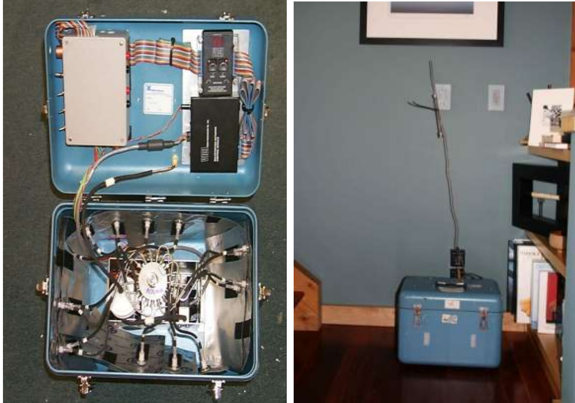
Figure 5: The programmable active tracer gas sampling device. The picture on the left side shows detail of the sampling manifold and installed sample bags. The installed sampler is shown on the right, with the inlet to the instrument mounted to the top.
