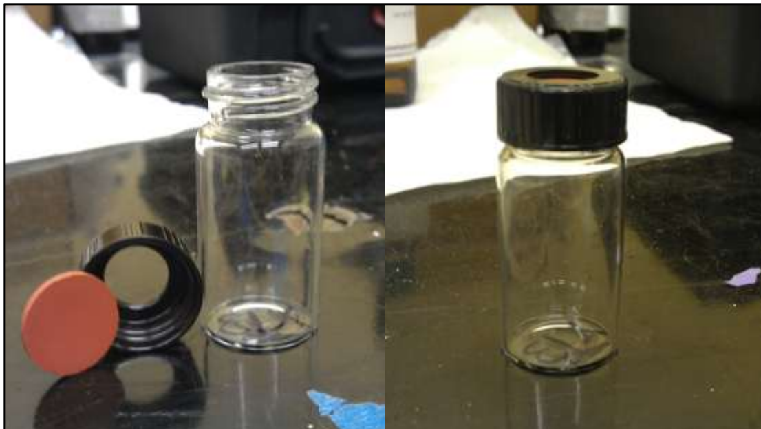
Figure 1: Emission vial for PFT sources. The photo on the left shows the vial cap and rubber septa insert separated. The photo on the right shows the assembled vial with septa inserted into the vial cap.
