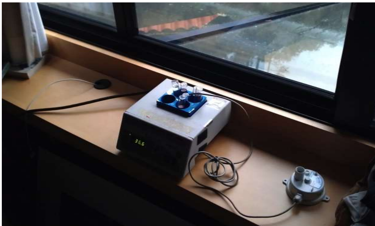
Figure 7: A dry block heater used to keep the PFT sources at a constant temperature. The tracer vials can be seen placed upside down in the blue-colored aluminum block. The temperature logger is to the right of the heater.
