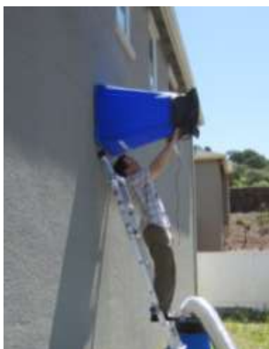
Figure 11: As this range hood outlet measurement shows, the ABT701's height requires the user to be well away from the terminal
