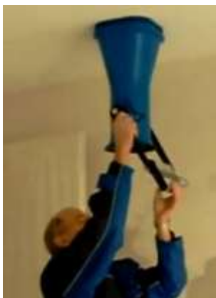
Figure 8: With the capture hood attached, the DIFF is more difficult to support with one hand
