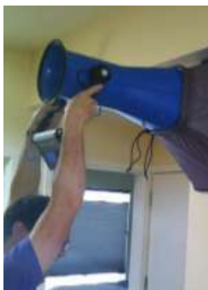
Figure 8: With the capture hood attached, the DIFF is more difficult to support with one hand
