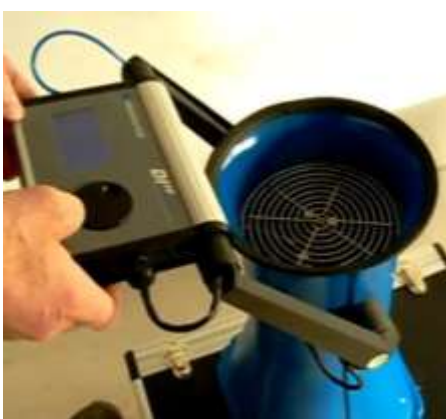
Figure 9: The DIFF's digital interface, with click wheel.
