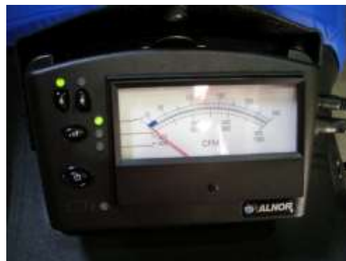
Figure 10: The ABT701's analog needle requires interpretation by its user so is susceptible to parallax error
