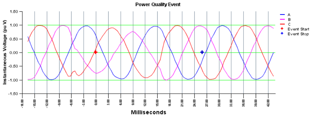
Figure 3a: 10/19/02 event voltage waveform, Block 1 (event 50182). 480V L-L monitor.
