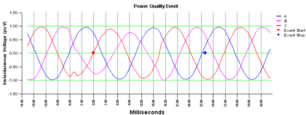
Figure 3b: 10/19/02 event voltage waveform, Block 2 (event 1632). 480V L-L monitor.
