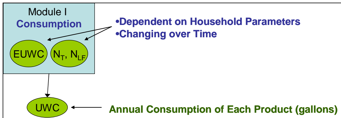
Figure 2 – Module 1 of the NWS Model. EUWC = end-use water consumption; N T = number of toilets; N LF = number of lavatory faucets; and UWC = unit water consumption.
