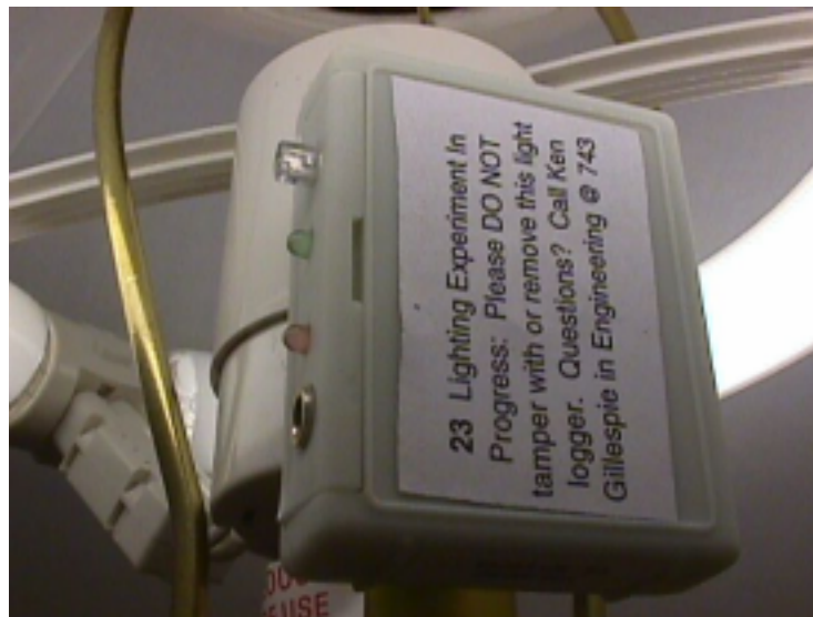
Figure 4: Lighting loggers were connected to all lighting fixtures in the experimental guestroom, including this table lamp.
