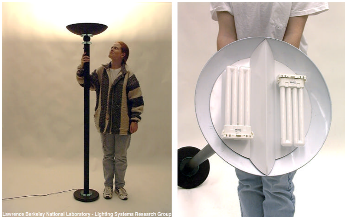
Figure 1. Example of a prototype torchiere design. The reflector and lamp configuration shown on the right is similar to the design of prototypes one through five and nine.
