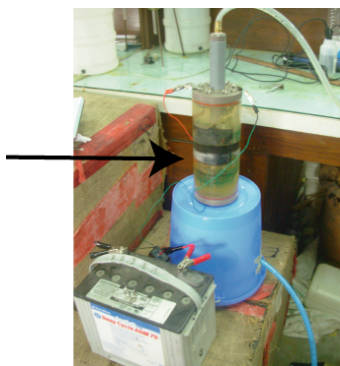
Figure 3: ECAR prototype device (shown by arrow) being tested at Bangladesh University of Engineering and Technology (BUET), in Dhaka, Bangladesh. Notice the 12V car battery - in the field, batteries could be coupled with solar photovoltaic panels.
