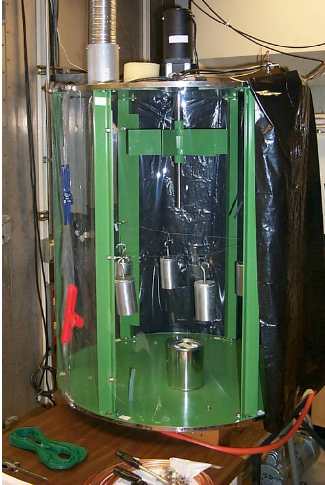
Figure 2 Chamber developed to calibrate passive samplers showing several samplers in the chamber along with a control (in can).
