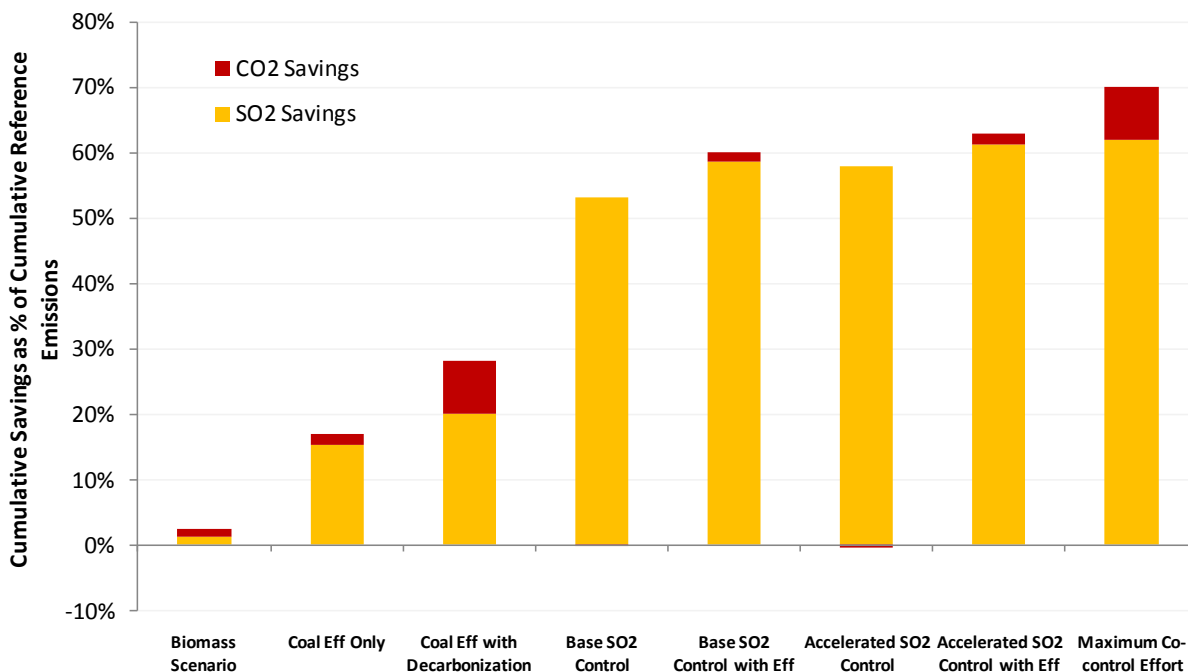
Figure ES-6 2005-2030 CO 2 and SO 2 Relative Emissions Reduction Potential of Co-control Scenarios
