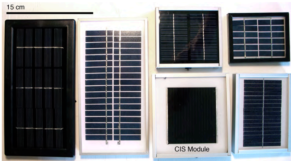
Figure A1: Various PV modules that are typical of those included with off-grid lighting products.
