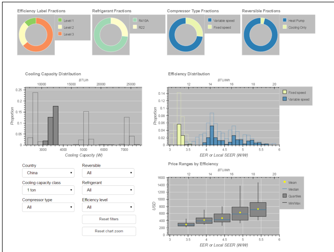
Figure 3. A visualization of the Chinese mini-split market, for the same era as shown in Figure 2, but with a filter applied to show only units having cooling capacity of approximately 1 refrigeration ton. A much clearer relation between price and EE is apparent when the confounding factor of cooling capacity is controlled for.
