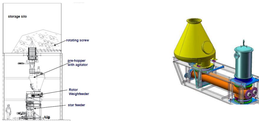
Figure 32. Rotor weighfeeders (left) and screw weighfeeders (right) for dosing solid waste fuels (Leong 2008; Schenck Process 2009)
