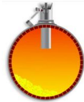
Figure 33. Cadence’s mid-kiln fuel injector technology (Cadence 2012a)
