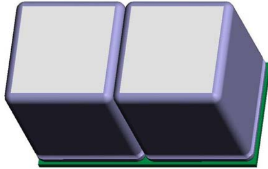
Figure 2-10 Representative Voltage Stiffening Brick from cubic electrolytic capacitors.
