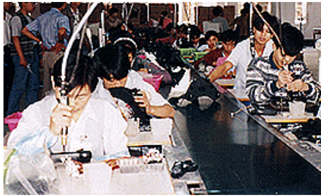
Figure 1-3 Manual assembly of power electronic converters [6].
