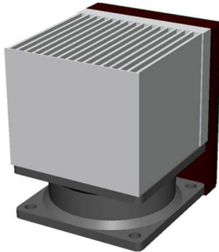
Figure 2-3 Representative air-cooled Power Switching Brick (1 of 2).
