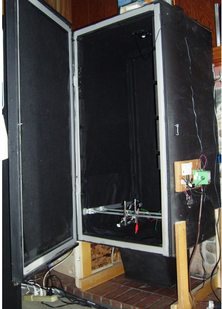
Figure 9. Inside Dark Box. The mounting devices for the flashlight is located on the bottom end of the box, the illuminance meter is mounted on the opposite end and the datalogging equipment is mounted on the exterior of the box (right-hand side)
