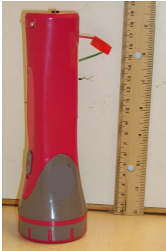
Figure 3-4. Flashlight B. Rechargeable 4 LED flashlight with a 800 mAh rated battery.
