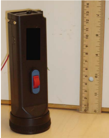
Figure 1-2. Flashlight A. Rechargeable 3 LED flashlight with a 1000 mAh rated battery.
