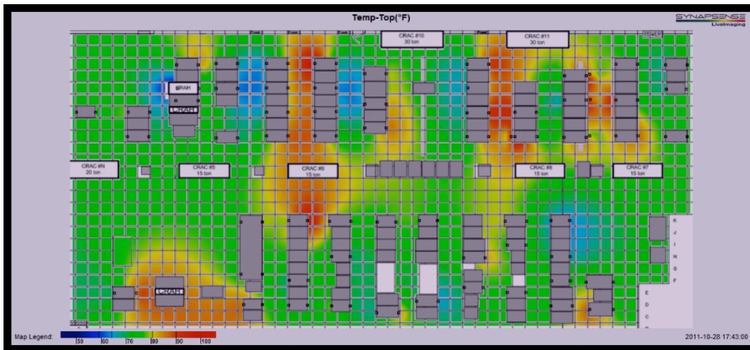
Figure 19. Rack Top Air Intake Temperature Map at 5:00pm, October 28, 2011
