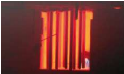
Figure 37. Testing of a high-temperature membrane module on a furnace; view from the stack through the module into the furnace (BFI 2009/2010)
