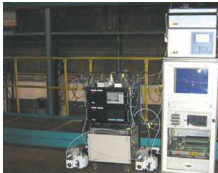
Figure 40. Modified burn-out measuring system during industrial trials on a hot-dip galvanizing line (BFI 2009/2010)
