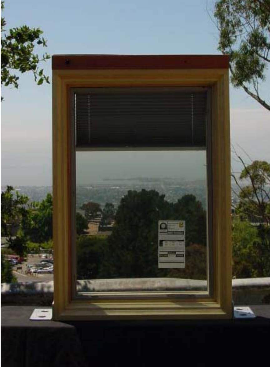
Figure 2: Prototype Window (Shades in the process of closing to respond to direct solar radiation)
