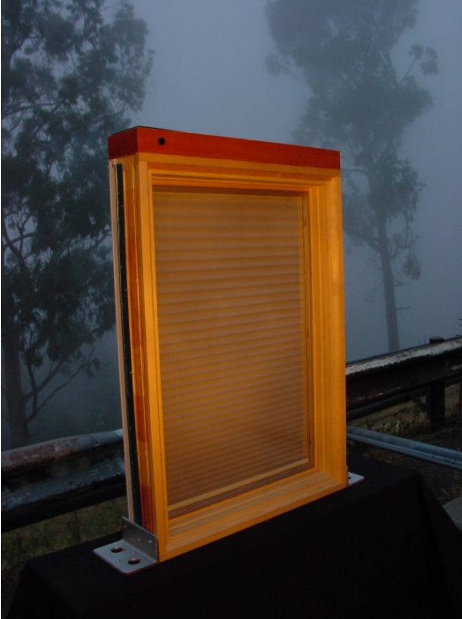
Figure 5: Prototype Dynamic Window at Dusk (Shades closed for privacy and increased insulation)
