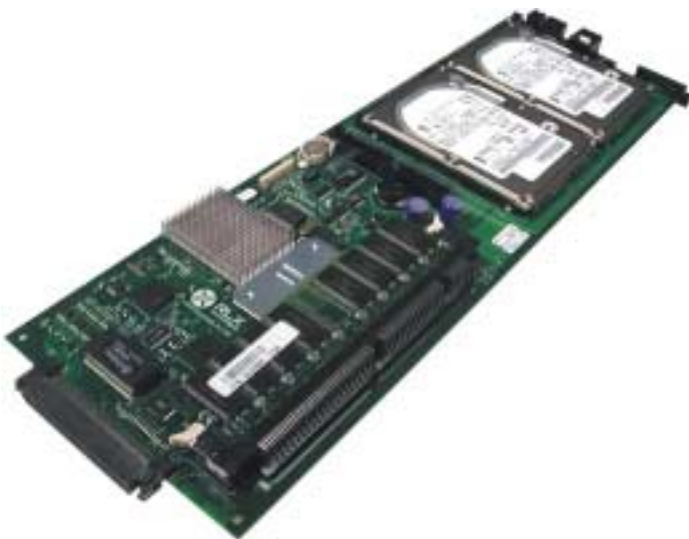
Figure 15 Typical Blade server Source: RLX Technologies
