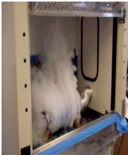
Figure ES-4. High-performance Berkeley Hood, showing full pollutant containment during flow-visualization test.
