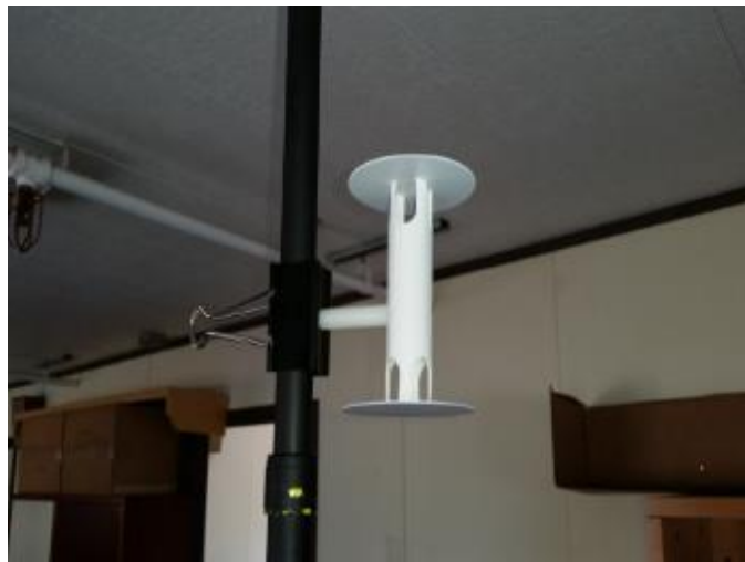
FIGURE 8. THE RADIATION SHIELD FOR THE AIR TEMPERATURE SENSORS
