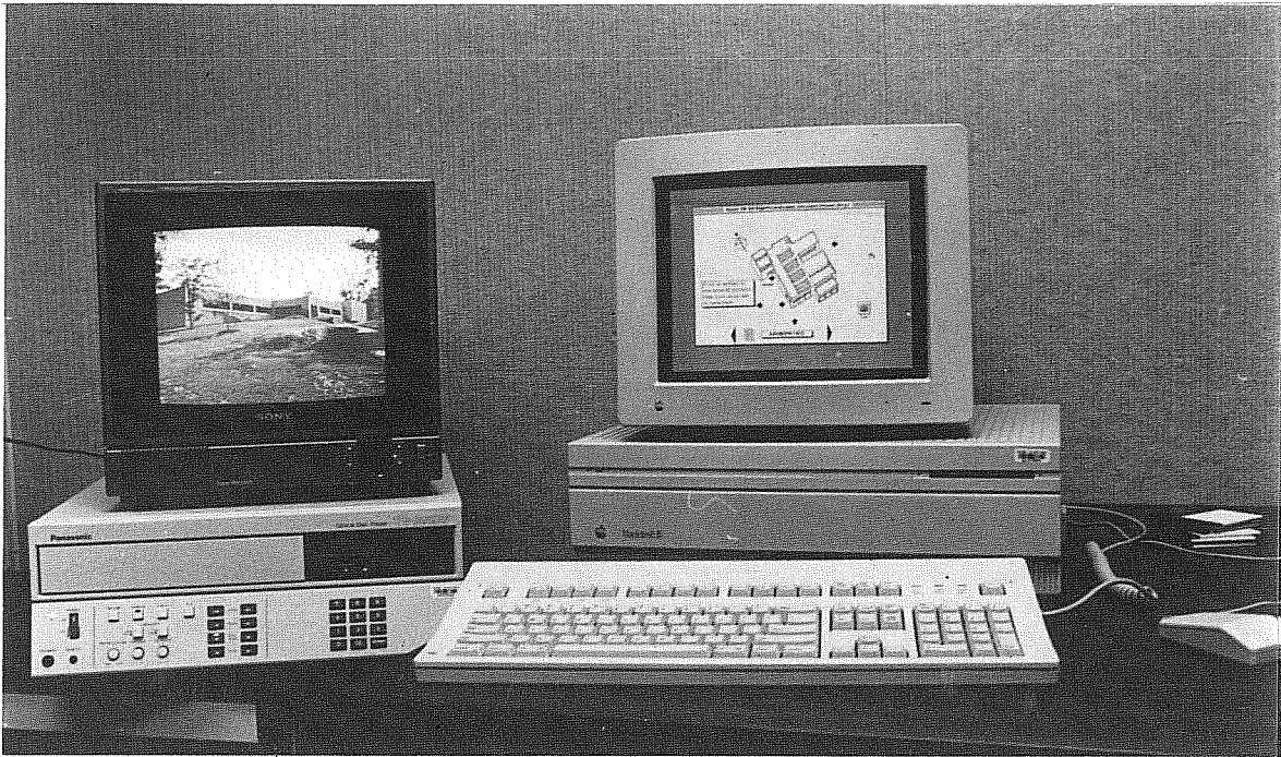
Fig. 4. A building tour of Mt. Airy Library. The user clicks an arrow pointing to the axonometric drawing for that view on the monitor. (XBB 894-3730)
