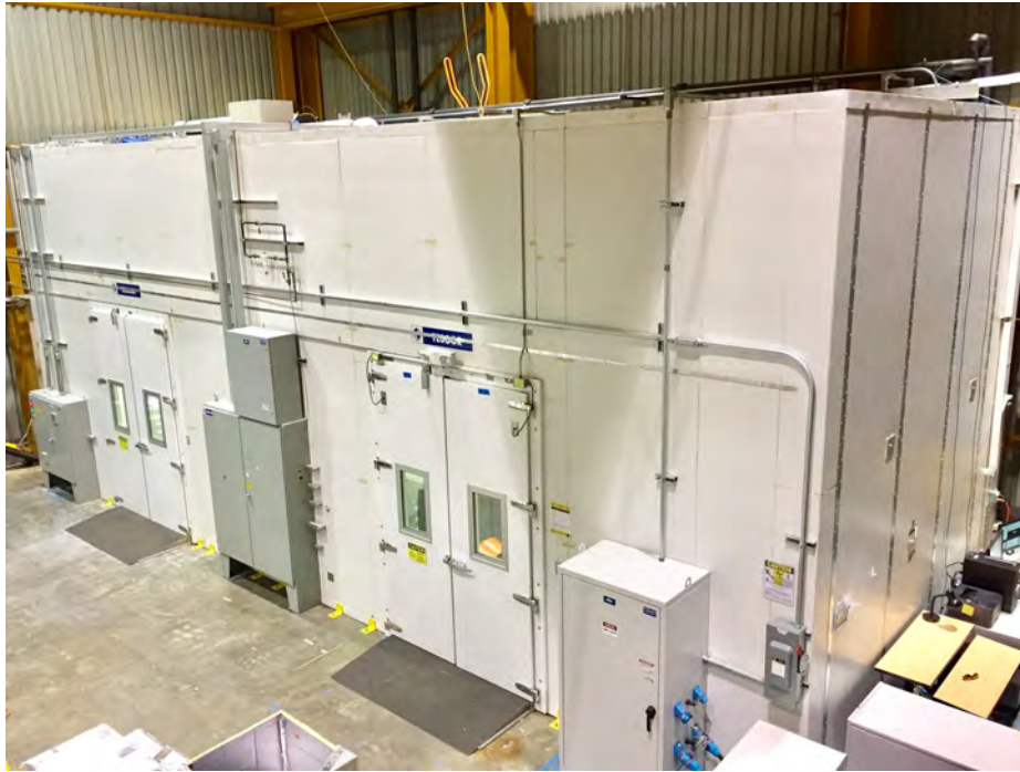
Fig. 4. A Photograph of LBNL's psychrometric test chamber.
