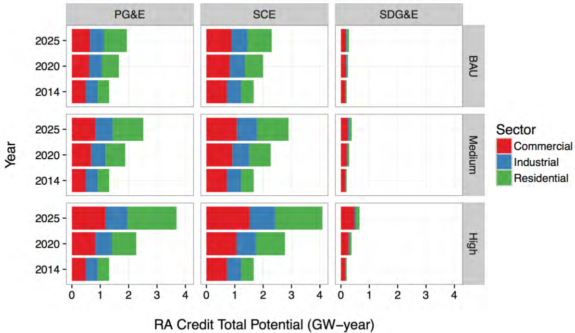
Figure 30: Cost competitive DR for each IOU service territory, by year, scenario and for each customer sector. The customer sectors are stacked bars depicting the cumulative DR potential (GW-yr) that fall beneath the price referent of $200/kW-year.
